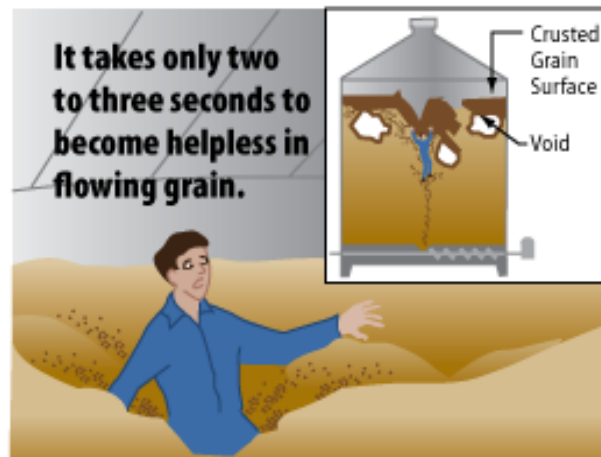
Figure III.5 Image of a Grain Engulfment Hazard
