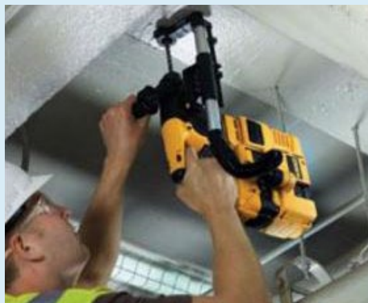
This rotary hammer has a built-in vacuum dust collection system. The drill bit is surrounded by a shroud that is attached to a vacuum to collect dust and bits of concrete. (Photo courtesy of DeWalt)
