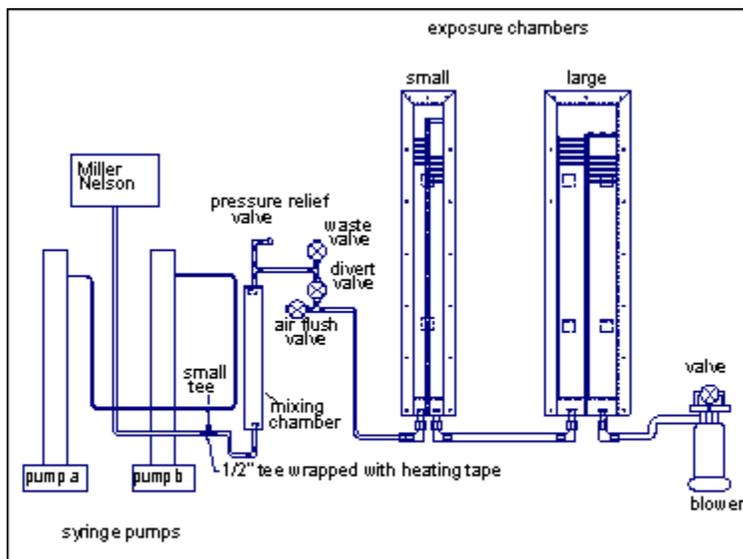
Figure 1. Test atmosphere generation and sample collection apparatus.
