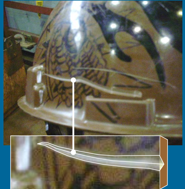
The edge of the steel plate that swung out dug a furrow into the shipfitter's hard hat
