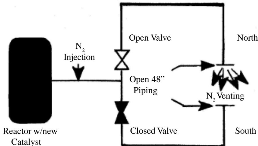
Note: Actual process/piping significantly more complex. N<sub>2</sub> injection point 150' and several stories in elevation from pipe opening .
