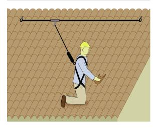
**Leave anchors in place**: Where practical, consider leaving roof anchors in place. It will make the current job simpler and reduce the burden for roofers in the future.
