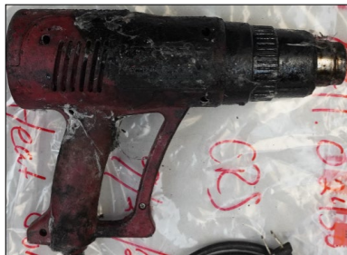
Heat gun recovered from fire (credit: US Chemical Safety and Hazard Investigation Board)
