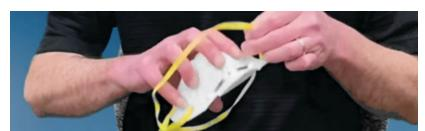
Inspect the respirator for damage. If it appears damaged or damp, do not use it.
