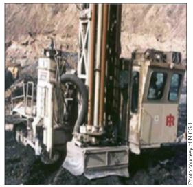
Vehicle-mounted drilling rigs with dust collection system around drill bit and low-flow water spray to wet the dust discharged from the dust collector. The enclosed operator's cab is on the right. The dust collection system is on the left.
