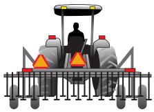
In 34 states, SMV emblems must be displayed on the rear of any tractor and its towed attachment traveling 25 mph or slower.
