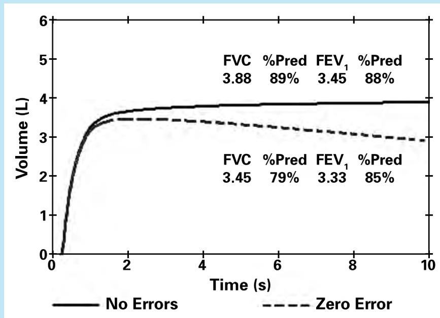
**Figure 8. Error: Zero-Flow Error Causing Flows to be Under-Recorded.** FVC is much more reduced than FEV<sub>1</sub>, falsely increasing the FEV<sub>1</sub>/FVC and possibly masking true airways obstruction. Block the sensor when the spirometer is zeroed and hold sensor still during subject testing to avoid this problem.
