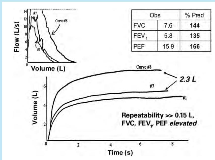
**Figure 5. Error: Sensor Contaminated or Blocked by Condensation, Mucus, or Fingers.** DELETE THIS TEST. The last curve (#8) shows the impact of blockage or contamination of the sensor after the 7<sup>th</sup> maneuver was recorded. The FVC and FEV<sub>1</sub> values are falsely increased on curve #8, exceeding values from the earlier maneuvers (curves #1 and #7) by more than 0.40 L. Technicians must replace the sensor if it becomes contaminated during the test.
