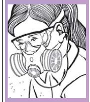
Half-mask respirators with chemical cartridges offer protection from breathing in chemical vapors.
