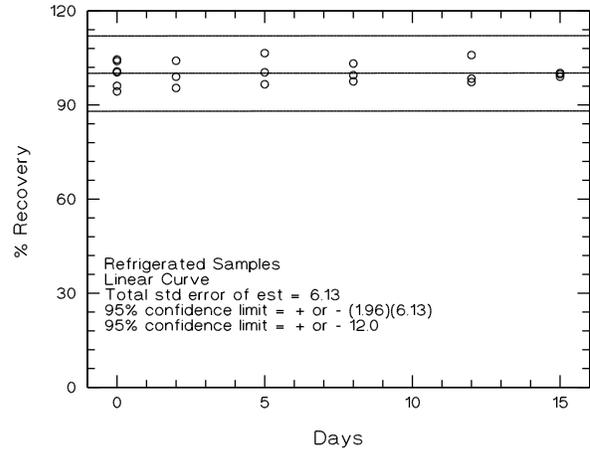
Figure 4.5.2. Storage test at reduced temperature (5°C).
