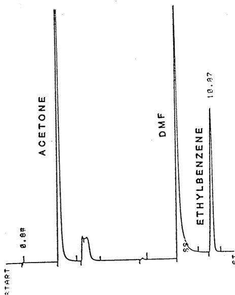
Figure 3.5.1. Chromatogram of acetone at the target level on packed column. Conditions are as described in Section 3.5.1.
