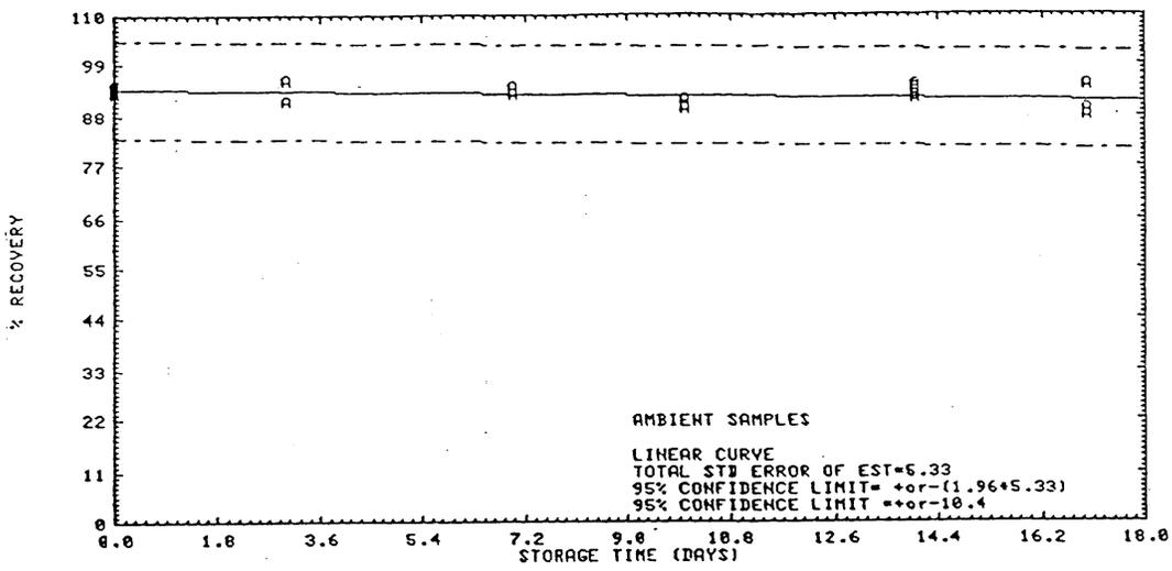
Figure 4.5.1.1. Acetone collected on Carbosieve S-III at 5% R.H. and stored at ambient temperature.
