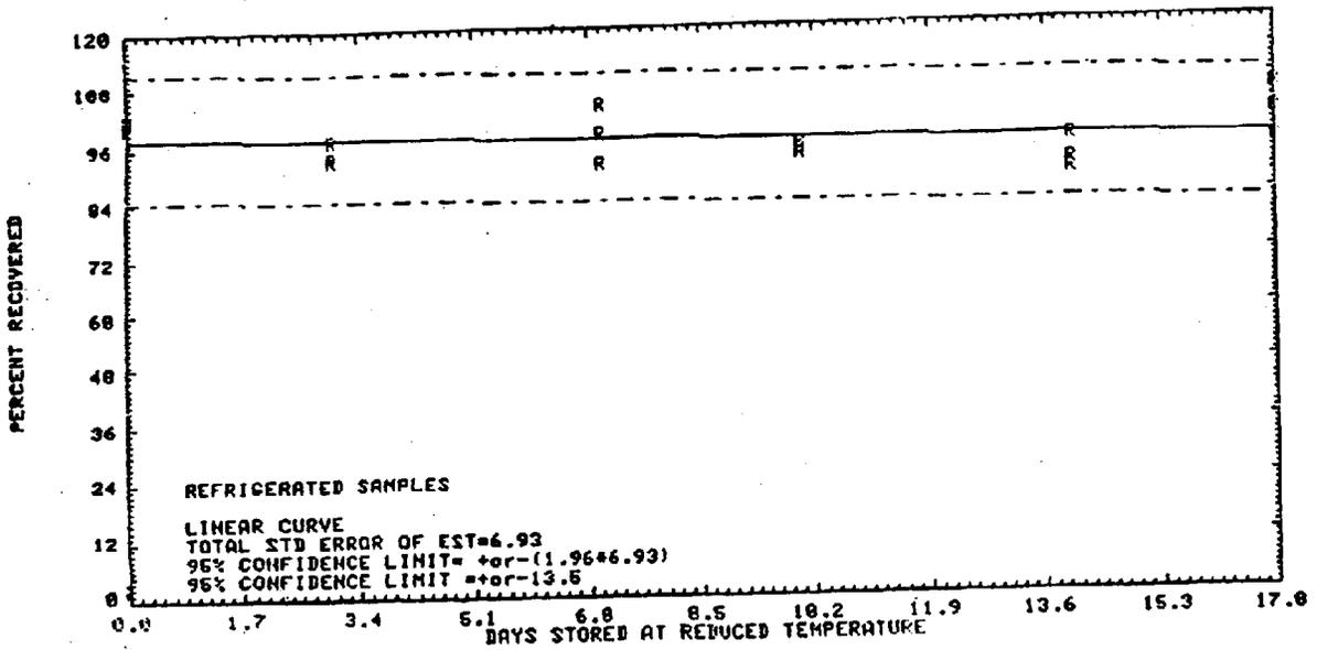
Figure 4.7.1. Refrigerated temperature storage test for EGDN.
