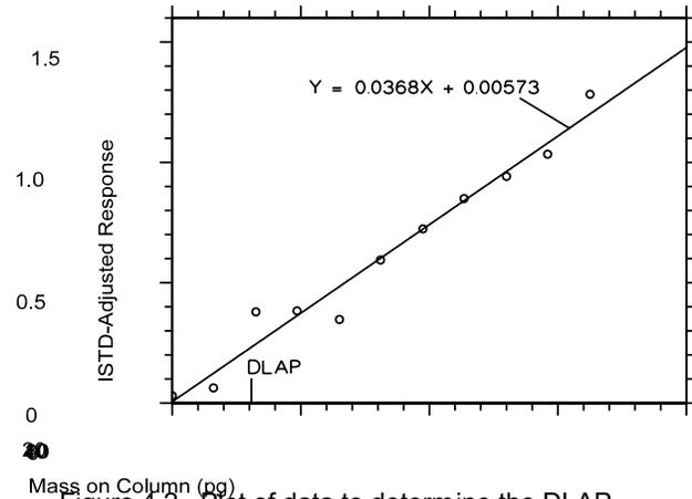
Figure 4.2. Plot of data to determine the DLAP.
