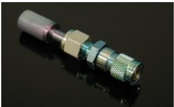
Figure 2.1.2.1 Short-term sampling orifice.
