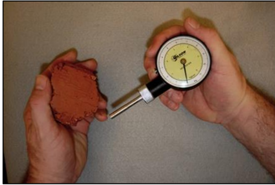
Figure 3.4.1.2. Flat face of sample ready for testing.
