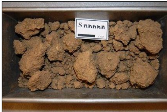
Figure 3.4.1.1. Ideal photo of an excavation sample.
