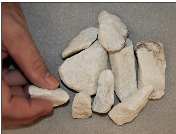
Figure 3.4.1.4. Angular gravel has relatively flat faces and generally sharp interfacial angles.
