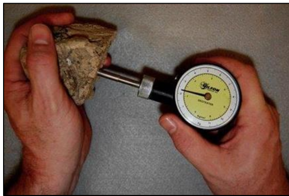
Figure 3.4.1.3. Testing with a penetrometer.
