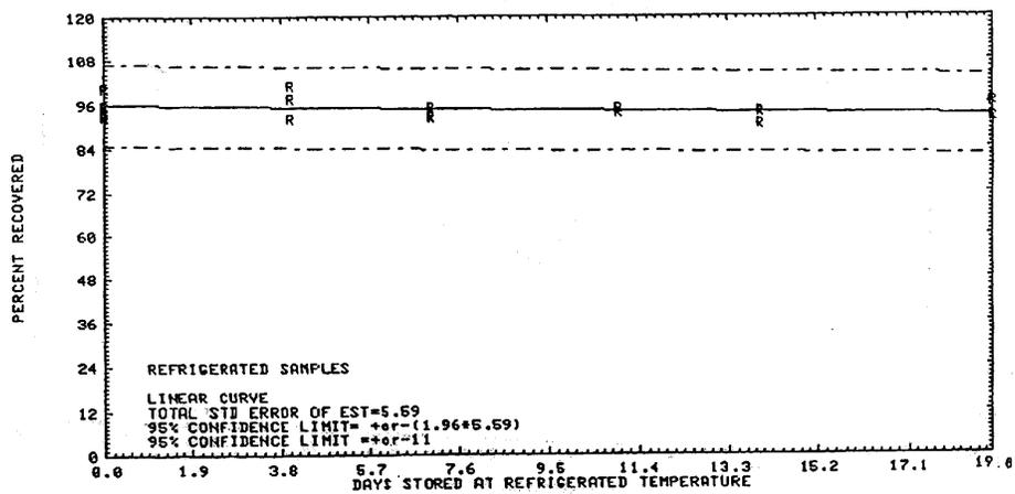
Figure 4.5.2. Refrigerated temperature storage test for valeraldehyde.
