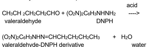
Initial laboratory experiments showed that glass fiber filters coated with DNPH were also effective for the collection and derivatization of valeraldehyde. Three coated filters were required for adequate sampler capacity. It is necessary to provide more sampler capacity for valeraldehyde than for the other two aldehydes because the PEL for valeraldehyde is 50 ppm while those for glutaraldehyde and crotonaldehyde are 0.2 ppm and 2 ppm, respectively.
