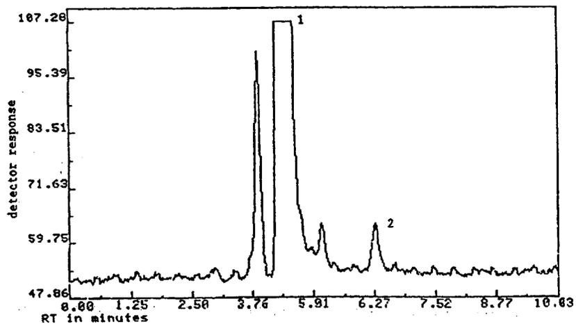
Figure 4.1. Detection limit of the analytical procedure for valeraldehyde. Peak identification was as follows: 1, DNPH; 2, valeraldehyde-DNPH.
