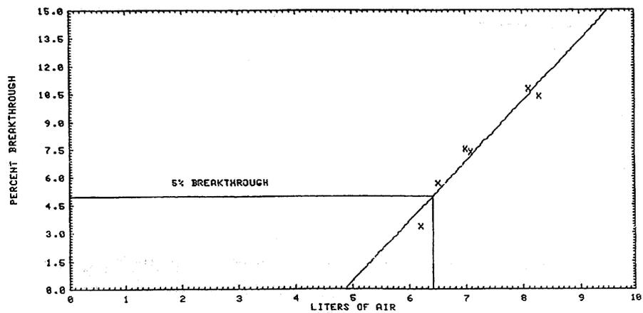
Figure 4.9. Sampler capacity for valeraldehyde.
