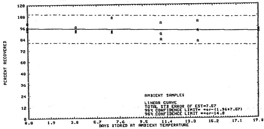
Figure 4.5.1. Ambient temperature storage test for valeraldehyde.
