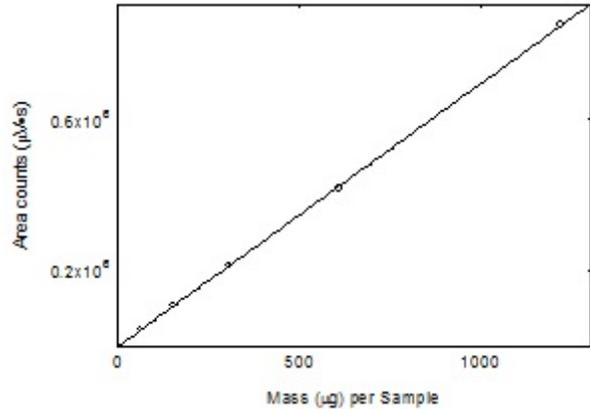
Figure 3.5.3 Calibration curve of benzyl acetate. (Y = 694 x - 336)
