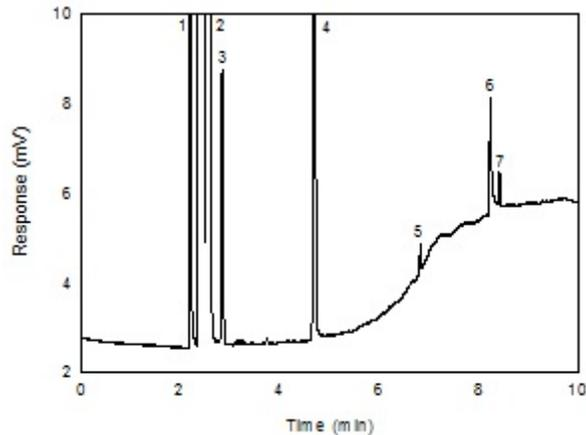
Figure 1.2.2. Chromatogram of the RQL of benzyl acetate. (1, 5, and 6 = impurity; 2 (doublet)= carbon disulfide; 3= benzene (contaminant in the carbon disulfide); 4 = *p*-cymene; and 7 = benzyl acetate)
