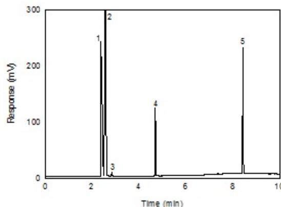
Figure 3.5.1. A chromatogram of 610  $\mu$ g/mL benzyl acetate in carbon disulfide with 0.25  $\mu$ L/mL *p*-cymene internal standard. Key: (1) and (2) carbon disulfide; (3) benzene contaminant in the carbon disulfide; (4) *p*-cymene; (5) benzyl acetate.
