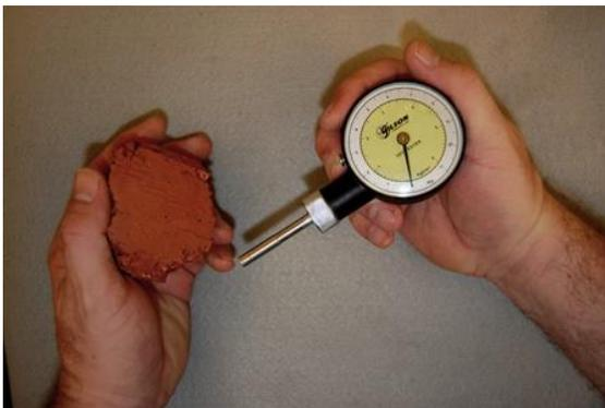
Figure 3.4.1.2. Flat face of sample ready for testing.
