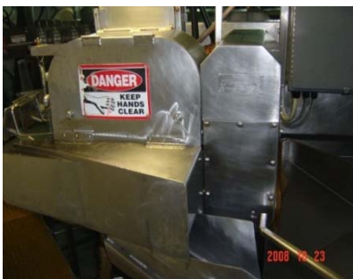
Guard with appropriate signage
