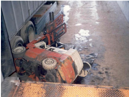
Photo: overturn after driven off dock, seat belt not worn, fatality
