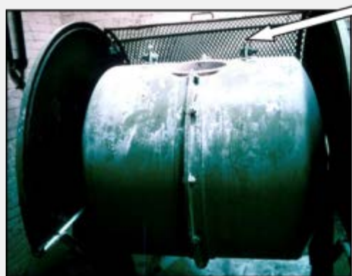
Interlocked guard on revolving drum
