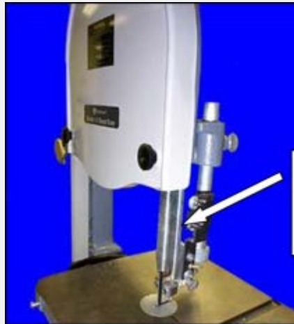
Bandsaw blade adjustable guard
