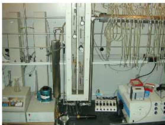
Figure 2. Sample exposure apparatus with small exposure chamber.
