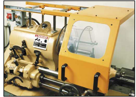
Machine guards must be kept in place for the employee's protection.
