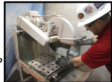
*Water flow rates must be sufficient to minimize visible dust.*
