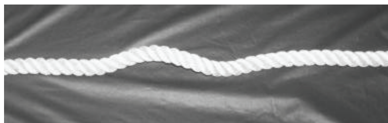
Figure D-024 Corkscrew Due to Twist
