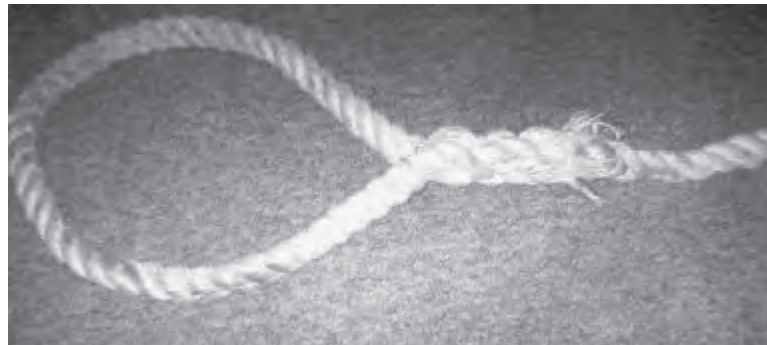
Figure D-018 3-Strand Splice of Poor Quality
