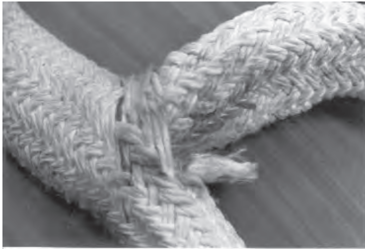
Figure D-020 Tearing at Leg Junction of Eye Splice
