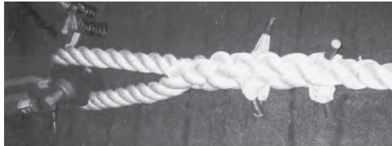
Figure D-017 Properly Made 3-Strand Eye Splice (correctly made – shown for reference)
