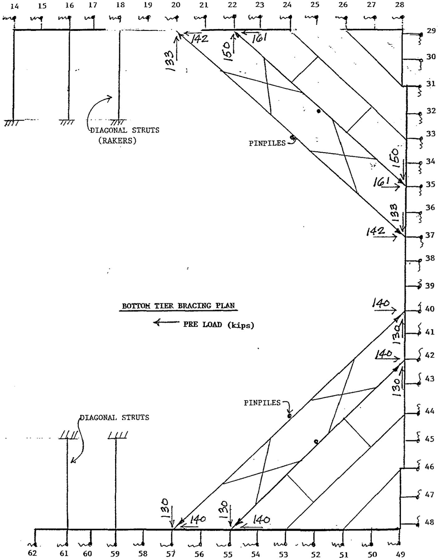
PRE LOAD OF THE BOTTOM TIER USED IN THE COMPUTER ANALYSIS
