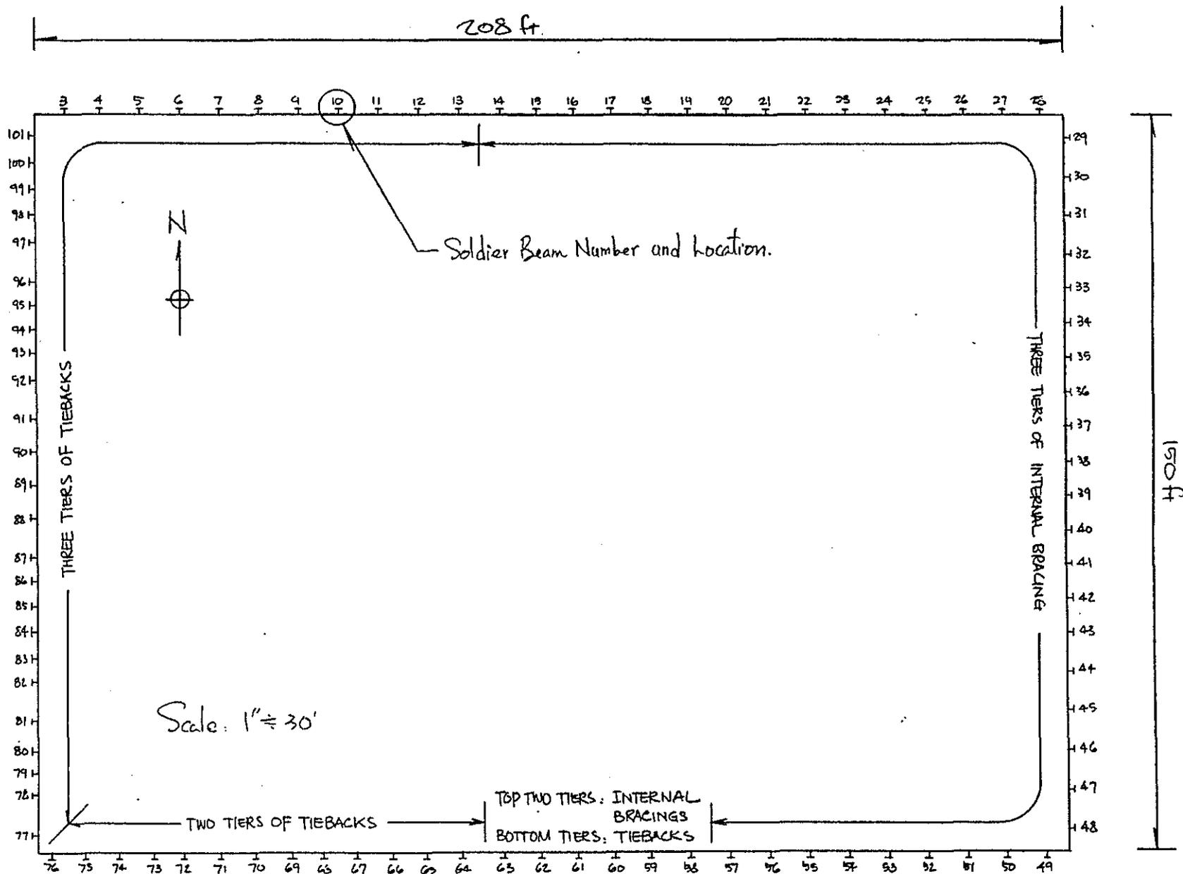
Figure 3.2 Plan Location of Soldier Beams in the Original Design Plan
