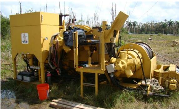
Figure 17 – Three Drum Hoist (Side)
