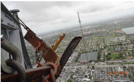
*Figure 25 – Bent Top Track Plate (provided by Stainless)*
