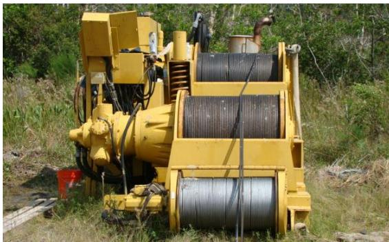
Figure 16 – Three Drum Hoist (Front)
