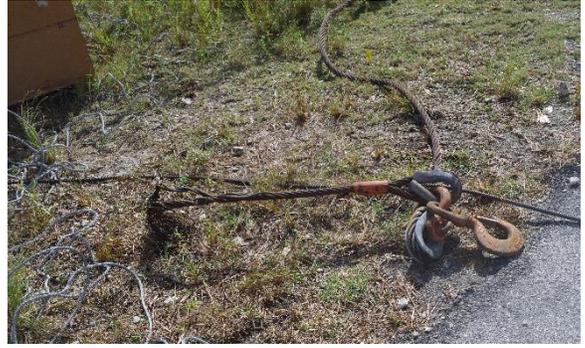
*Figure 23 – Fracture in Basket Sling*
