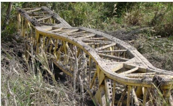
*Figure 14 – Gin Pole Section Break*
