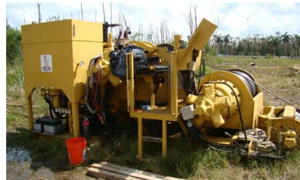
Figure 17 – Three Drum Hoist (Side)
