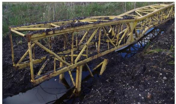
*Figure 15 – Rooster Head Section Buried*
