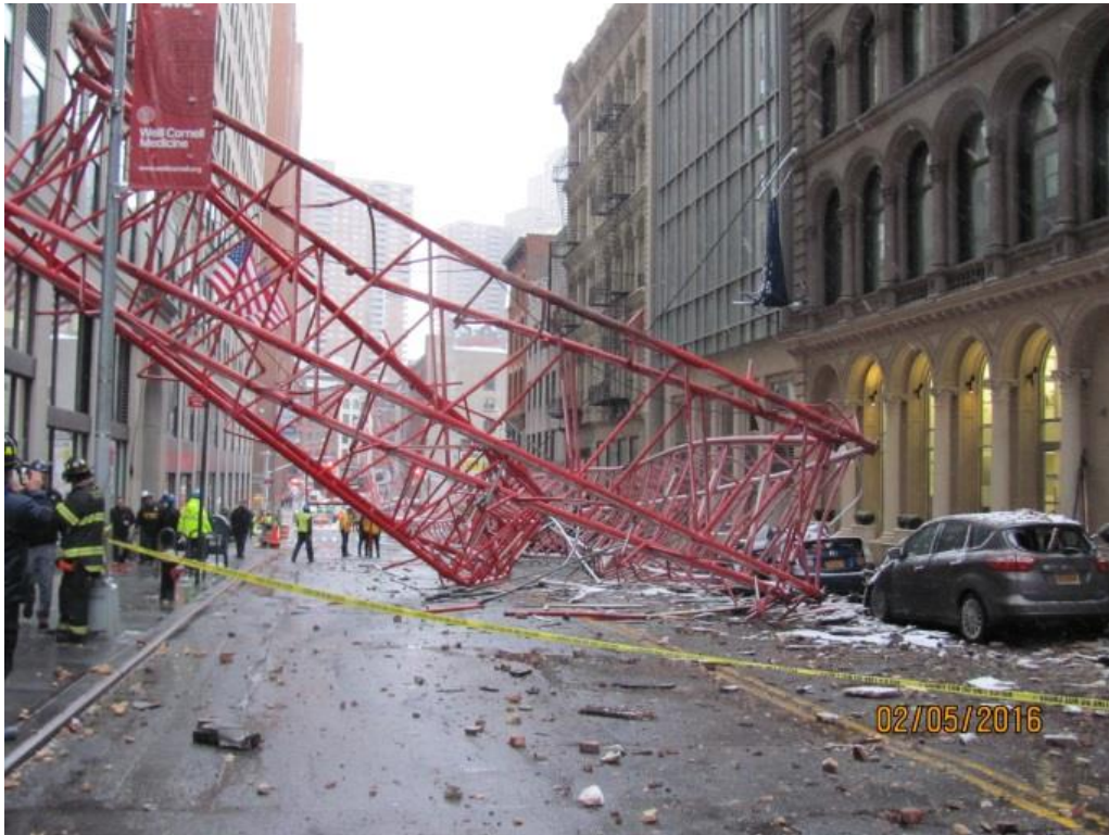
Figure 3 Jib head section after the incident – street view 1.
