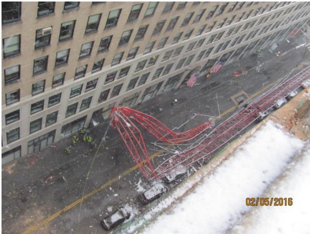
Figure 2 Jib head section after the incident – aerial view.
