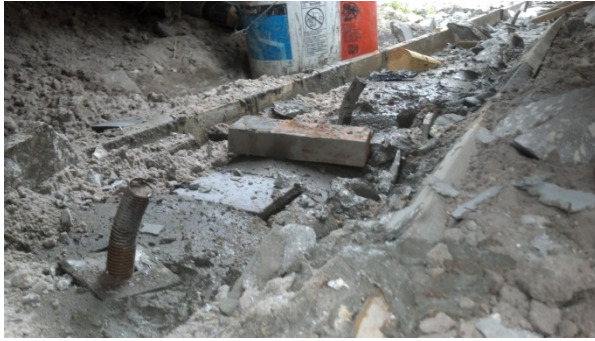
Fig. 24 Failed anchor bolts at the foundation
