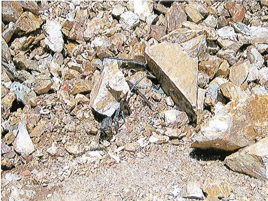
Figure 20 Type and Size of Rock Pieces at the Center of the Collapse.
