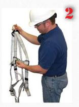
If chest, leg, and/or waist straps are buckled, release straps and unbuckle at this time.
