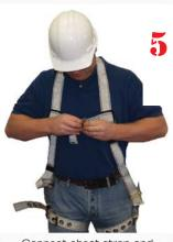
Connect chest strap and position in midchest area. Tighten to keep shoulder straps taut.
