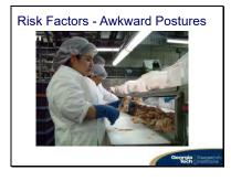
One of the more common postures we see that concern us is the wrist deviation above. Several things can cause this type of posture. In the picture above, it appears to be the orientation of the work and possibly the tool shape. The worker may be able to reposition the product that she is cutting to eliminate the deviation in her wrist. Selection of a tool that has a curved or pistol shaped handle could be might also be used to reduce the bending of the wrist.
