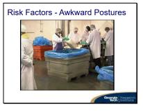
Here is another example of a wrist deviation. It is the dumping motion that is causing this posture. In this case, there is a good deal of force involved which would increase this worker's risk of developing a MSD. Items like the powered dumping mechanisms or some vacuum devices may work well to to alleviate this type of problem.
