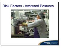
Here the worker is holding her arms still while the part is being cut by a circular saw. Her arms are almost fully extended. The saw is too high and too far away from the worker.
