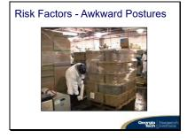
The worker here is wrapping the pallets with a plastic film. He is already leaning to one side slightly. As he gets lower on the pallet, the sideways leaning will get more pronounced as will the forward bending. Several companies have replaced this operation with an automatic pallet wrapper (palletizer). They have eliminated this operation altogether.
