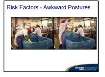
This is an example of the wrong tool and the wrong work station height. This gentleman is using a full size shovel to load products onto a work station. The bad combination is causing the worker to work with one hand over his head and with an uneven loading of the upper body (weight on one side of the body). Powered dumpers, vacuum transfer, better conveyors to deliver products, etc. may help or eliminate this hazard.
