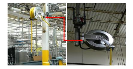
Solution: Elevated - retractable hose reels minimize trip hazards from hoses
