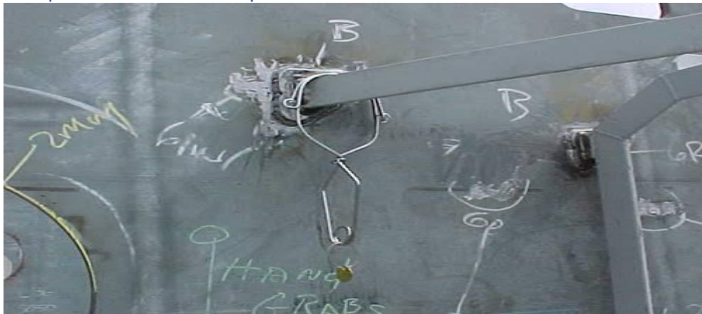
Hook provides 5000lb anchor point
