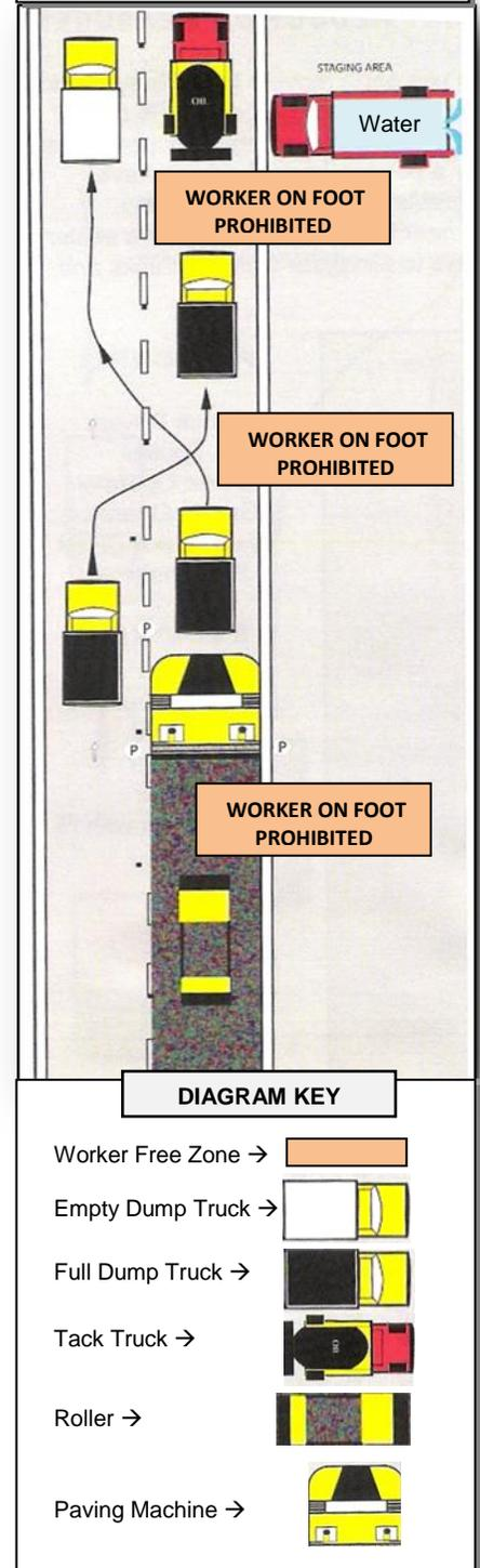
located as far as possible from vehicle paths. Parking, toilet, and break areas should be staged away from the principal conflict points involved with the paving rollers and dump trucks.
