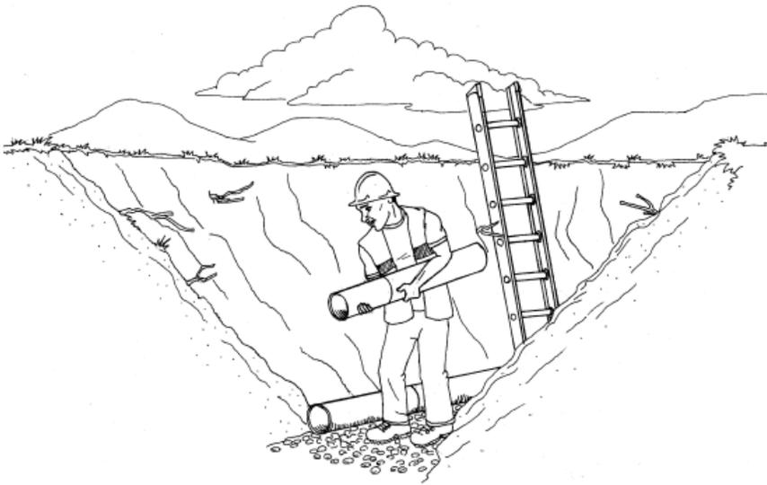
**Sloping:** The safe angle for the slope depends on the soil type.
