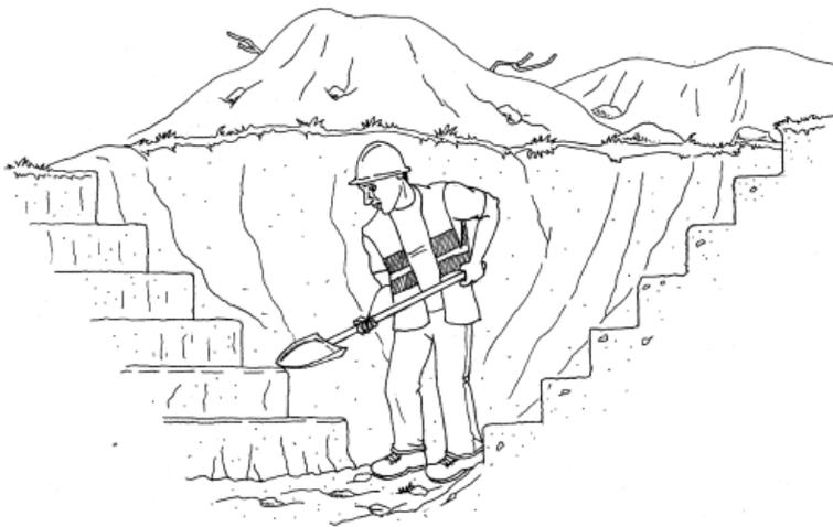
**Benching:** This is a safe method with Type A or Type B soil only.
