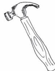
**Tool Safety:** Always make sure the head of the hammer is firmly attached to the handle so the head doesn’t fly off.
