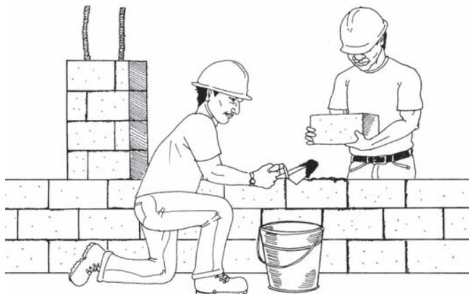
**Unsafe Work:** You must cap the ends of exposed “rebars” (reinforcing bars) if anyone can walk into them or fall onto them.
