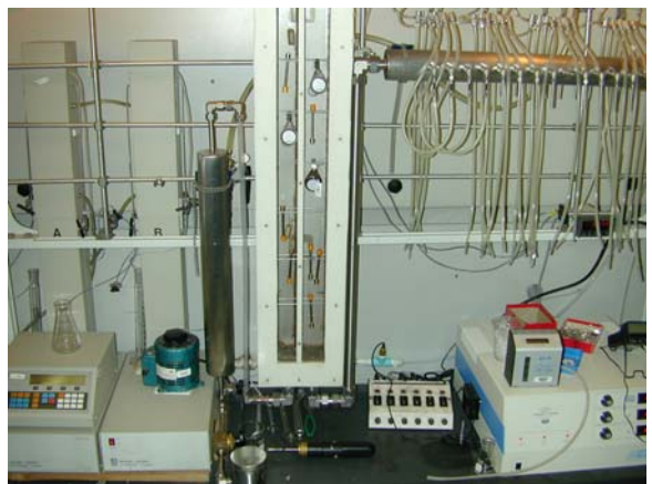
Figure 2. Diffusive sampler exposure apparatus with small exposure chamber.
