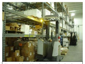
Upper rack is positioned at the same level as the overhead guard, preventing the possibility of an under-ride. The forklift shown in this photograph has an overhead guard and an extended backrest. Kits with additional posts are other safety features that are available on many forklifts.
