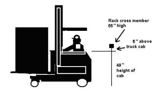
Drawing is not to scale. The small square on the body of the driver represents the approximate position of the rack cross-member after the accident.
