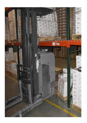
This photograph depicts a forklift under a storage rack after an under-ride accident. The crossbar is protruding above the operator's cab. Forklift manufacturers have various features available to assist in preventing such under-rides.
