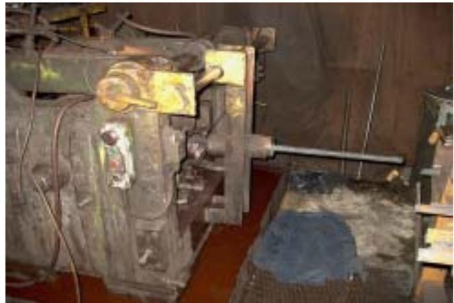
Figure 1: Bar Straightening Machine
