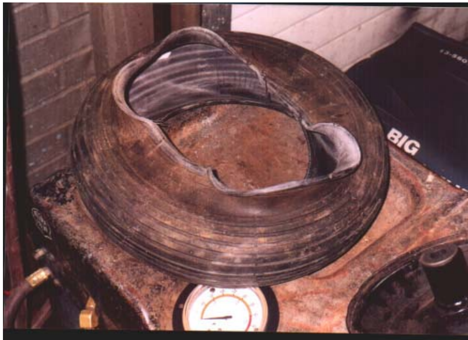
Picture depicting damage to tire that occurred during attempt to inflate a mismatched tire and rim
