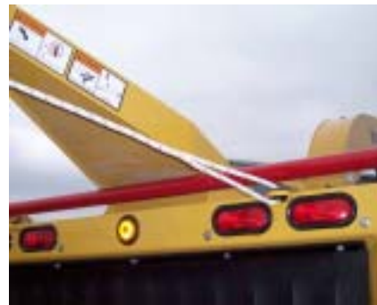
Winch line Safety Interlock and Storage Hook
