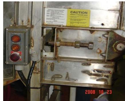
Example: Machinery, equipment, or system not capable of accepting a lock without retrofitting.
