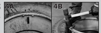
CURRENT PRODUCTION: THREE-PIECE SOLID RIM; SPLIT LOCK RING; SOLID FLANGE-M, CR, 5 DEGREE
