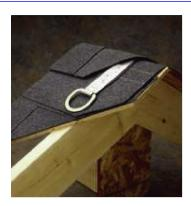
Retrofit with anchors: If the roof was not fitted with permanent anchors, employers can install them as the first phase of the job. This retrofit process should be planned so that the roof remains intact and does not leak after the job is completed. It will likely be necessary to replace an additional shingle or reset a couple shingles or tiles. If attaching a new anchor, roofers must fix it to the truss or rafter structure underneath. Roof sheathing does not provide enough support by itself.
