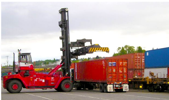
Top handler removing container from utility truck.
