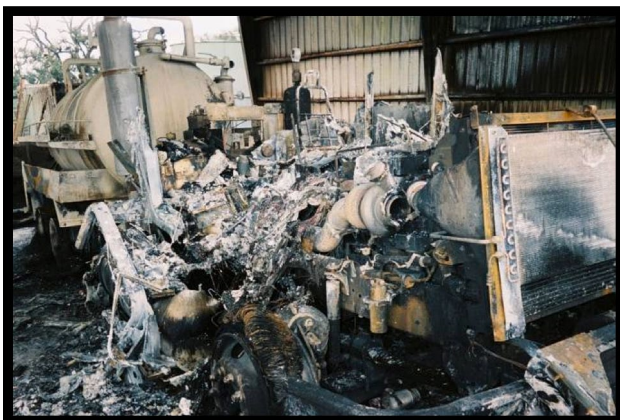
One of two vacuum truck diesel engines believed to be the ignition source for a fatal fire at an open air collection pit.
