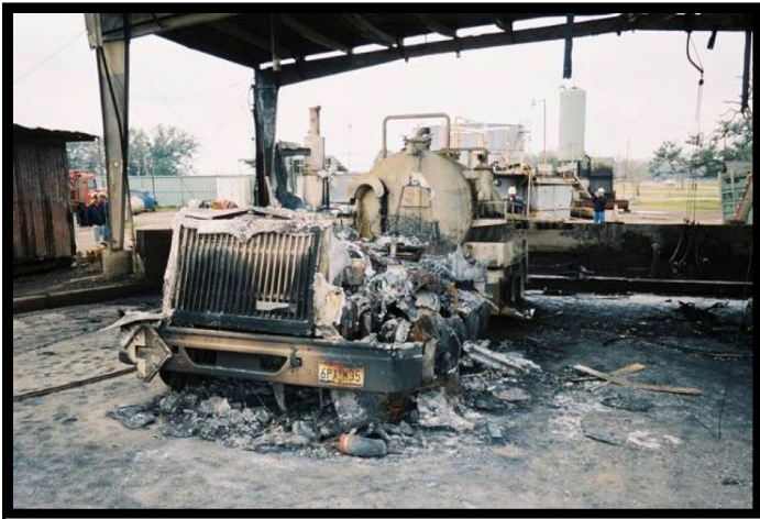
Three workers were killed and four injured in a fire resulting from a runaway diesel engine.
