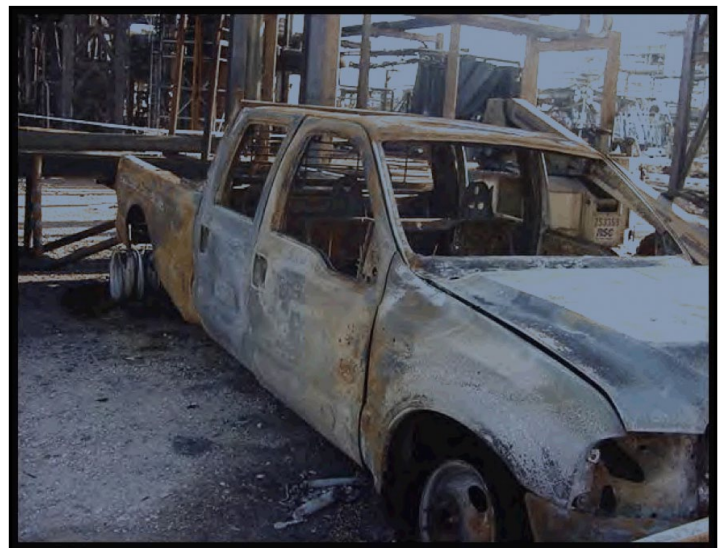
An idling diesel pickup truck believed to have ignited a vapor cloud from a nearby process area.
